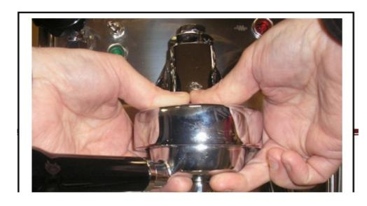
the gasket is up far enough then lock the portafilter into the group head and turn as far right as possible. Then remove the portafilter and re-install the insert basket and then
