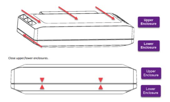
STEP C: Insert Two Screws in Lower Enclosure
