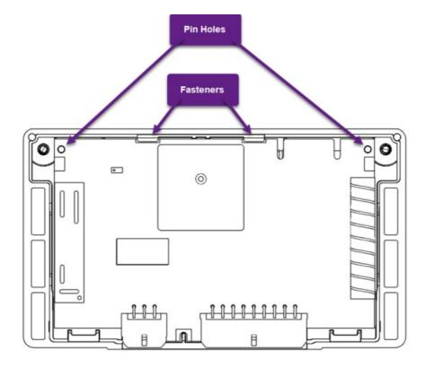
Swivel the PCB down into lower enclosure.
