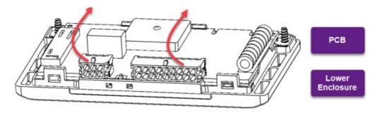
• Remove PCB from lower enclosure (to access battery in lower enclosure).
