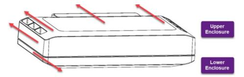
• Remove the upper enclosure from the lower enclosure (to view PCB).
