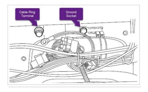
Connecting or soldering the unit to another ground wire is prohibited.
