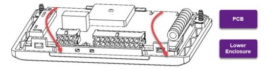
STEP B: Slide Upper Enclosure into Lower Enclosure
