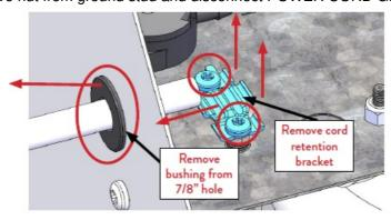
Remove the 2 screws holding the cord retention bracket using T25 Torx driver and remove retention bracket. Remove power cord and black bushing.
