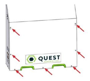
Remove 7 screws on access panel using T25 Torx driver, remove panel.
