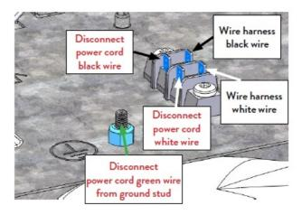
Disconnect POWER CORD BLACK wire from terminal Disconnect POWER CORD WHITE wire from terminal. Use 11/32" driver to remove nut from ground stud and disconnect POWER CORD GREEN wire from ground stud.
