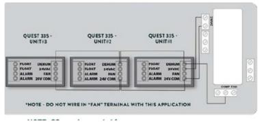
Remove the cover from the user interface to expose the terminal block inputs & outputs. Quest 335 Terminal Block Control Operations:
