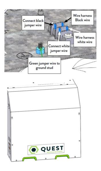
Replace access panel using T25 Torx driver to secure 7 screws.
