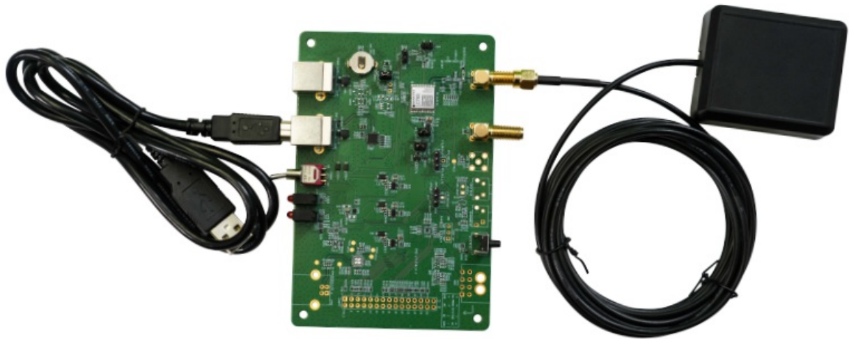
Figure 2: EVB and Components Assembly
