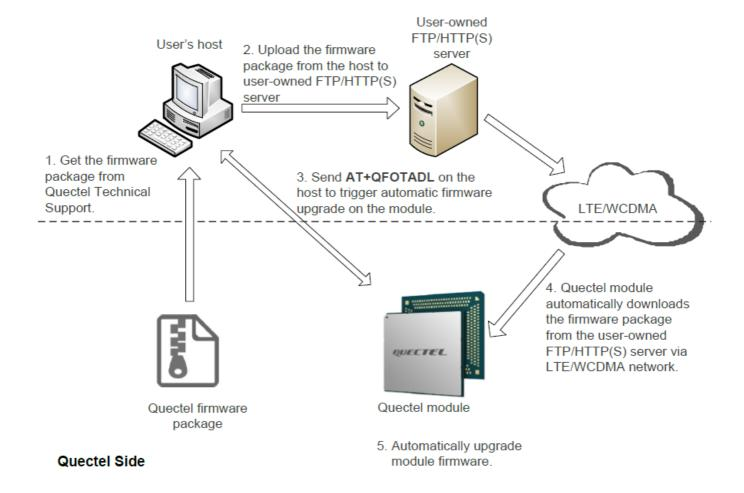
Figure 1: Firmware Upgrade Procedure via FOTA
