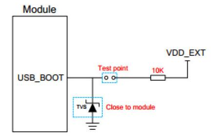
Figure 24: Reference Design of USB\_BOOT Interface
