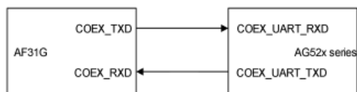
Figure 12: Coexistence UART Interface Connection
