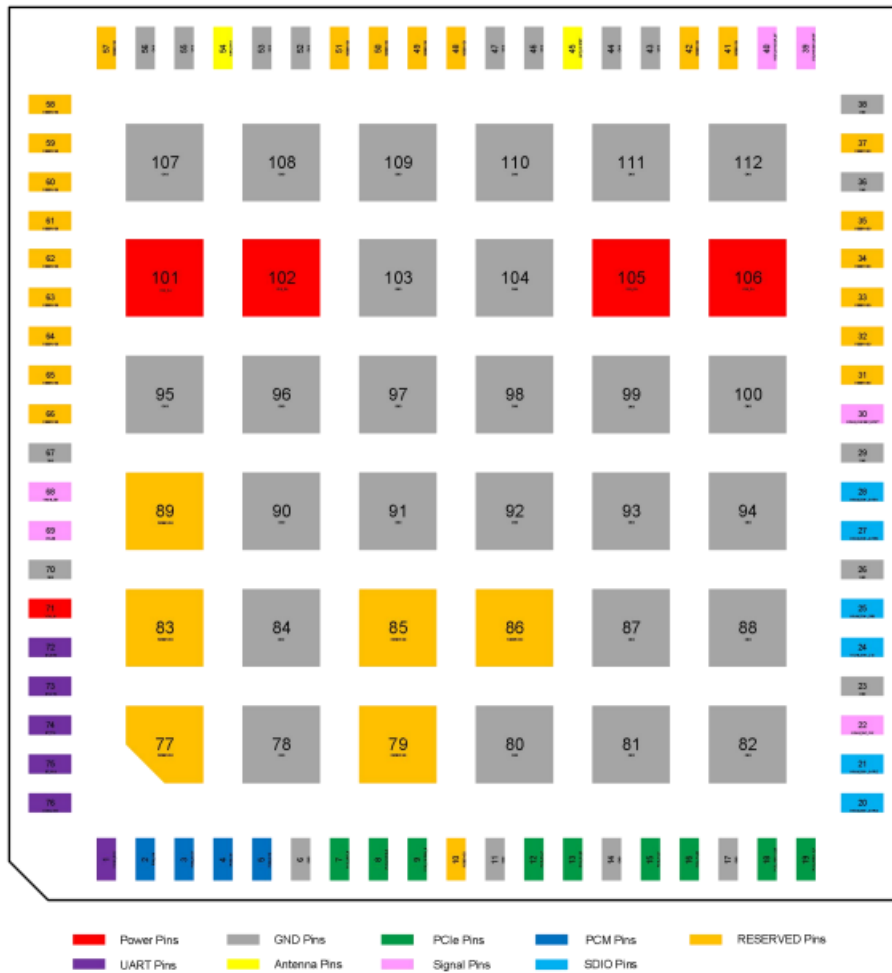
Figure 2: Pin Assignment (Top View)
