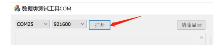
After opening the port, set delay time and data bytes to be sent
