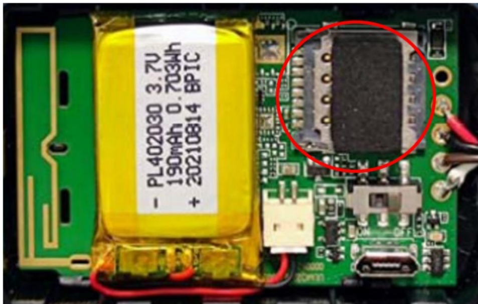
Figure 8. Installing a SIM Card
