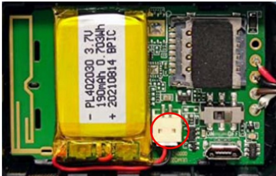
Figure 9. Installing the Internal Backup Battery
