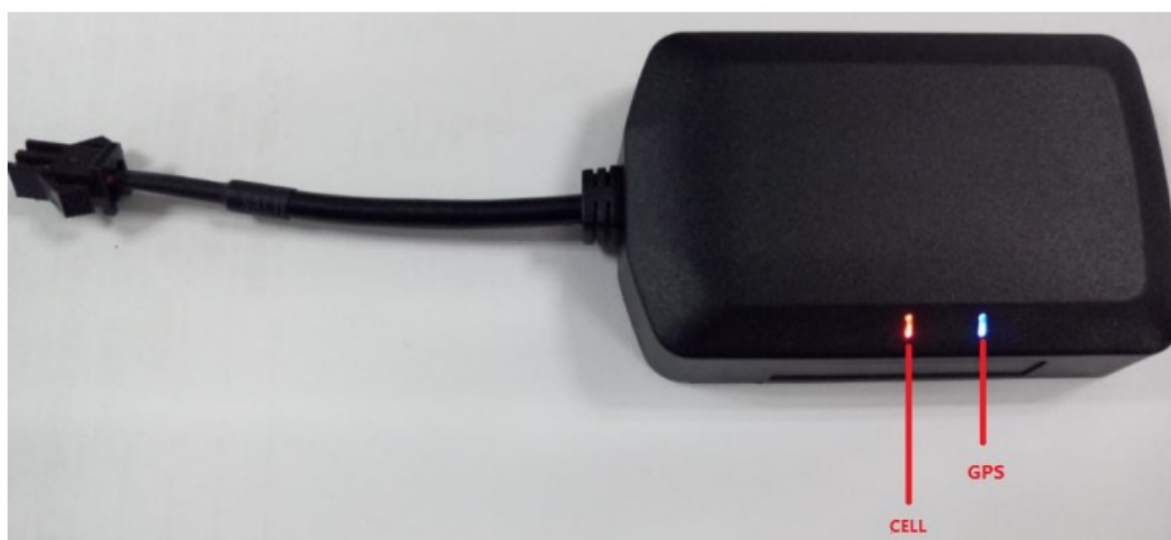
Figure 12. GV50(P) LEDs on the Case
