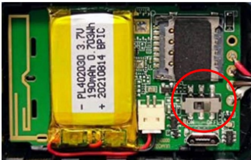
Figure 10. Switch and ON/OFF Position
