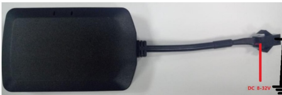
Figure 11. Typical Power Connection
