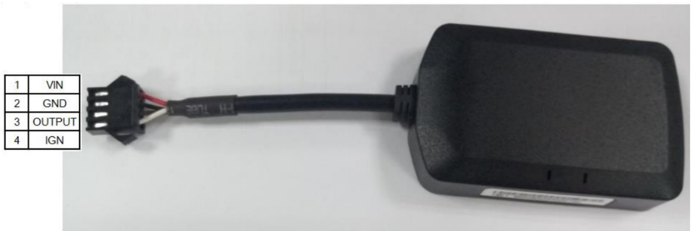
Figure 4. GV50P 4-Pin Cable Table 5. Description of 4-Pin Cable
