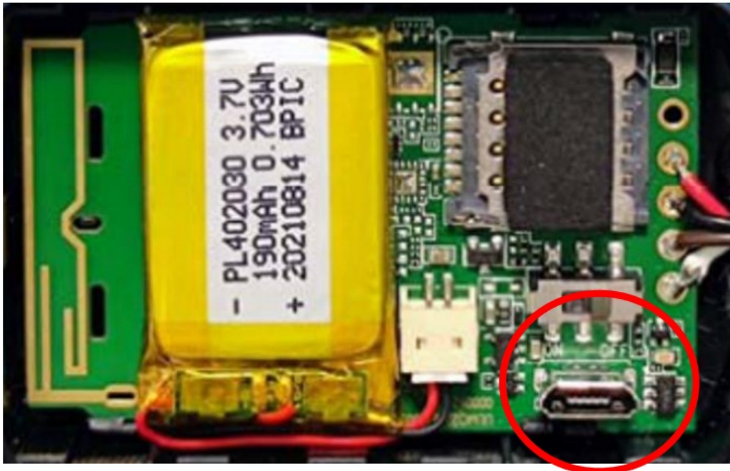
Figure 5. GV50(P) Micro USB Connector
