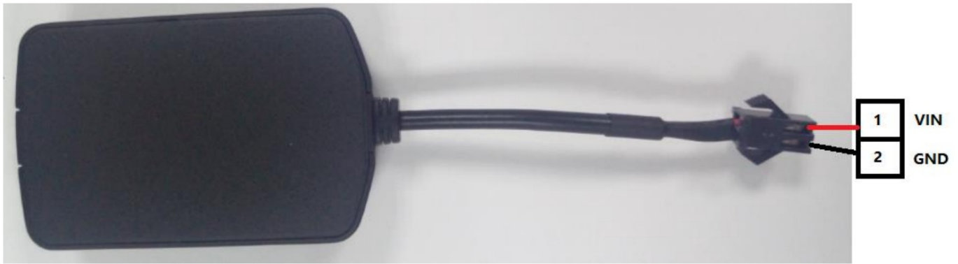
Figure 3. GV50 2-Pin Cable Table 4. Description of 2-PIN Cable
