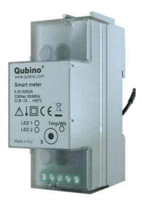
Smart Meter is an extremely versatile and powerful Z-Wave device for measuring energy in a single-phase electrical power network of up to 65A. A built-in microprocessor calculates energy, power and power factor from the measured signals. It is designed to be mounted on a DIN rail.
