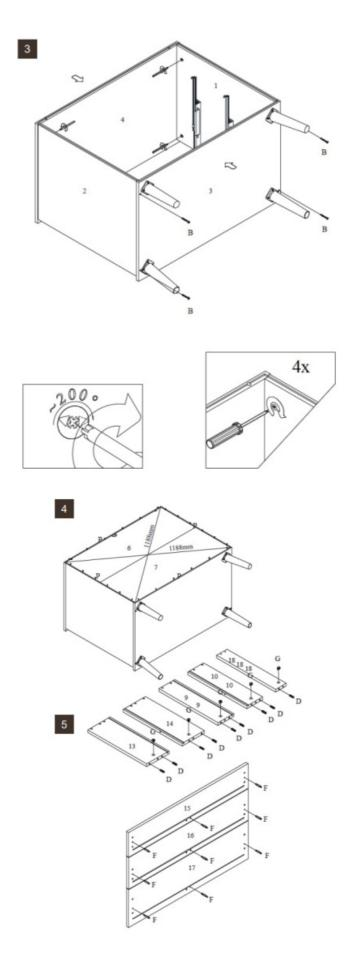
Be careful when installing the wood screws (P). They must be securely screwed into a panel.
