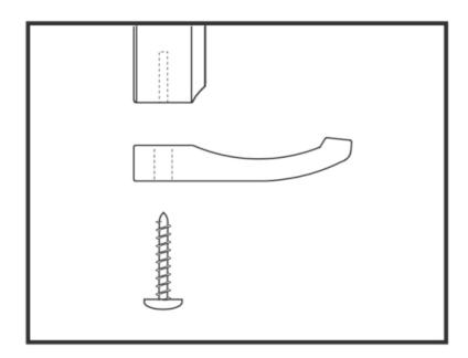
**Step 2:** Insert #8 x 1" truss head screws through holes in tray and into board frame. Tighten firmly.
