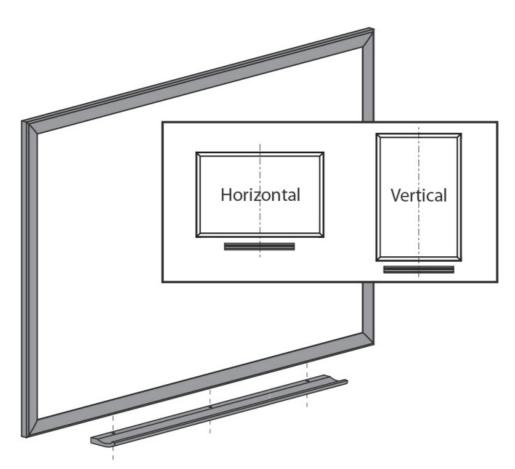
**Step 1:** Align holes in marker tray with pilot holes in bottom board frame Note: Pilot holes for tray are in long side of board only. Drill (3) 7/16" diameter pilot holes in short side of frame for vertical mounting.
