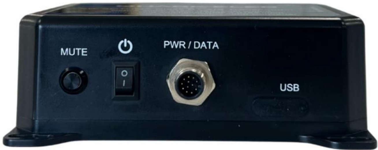
Figure 8 12 Pin power/data connector location
