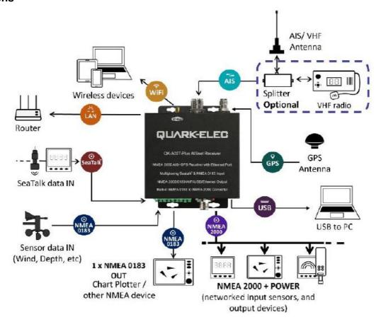
The A027+ NMEA 2000 AIS+GPS receiver has the following options for connection to other devices:
