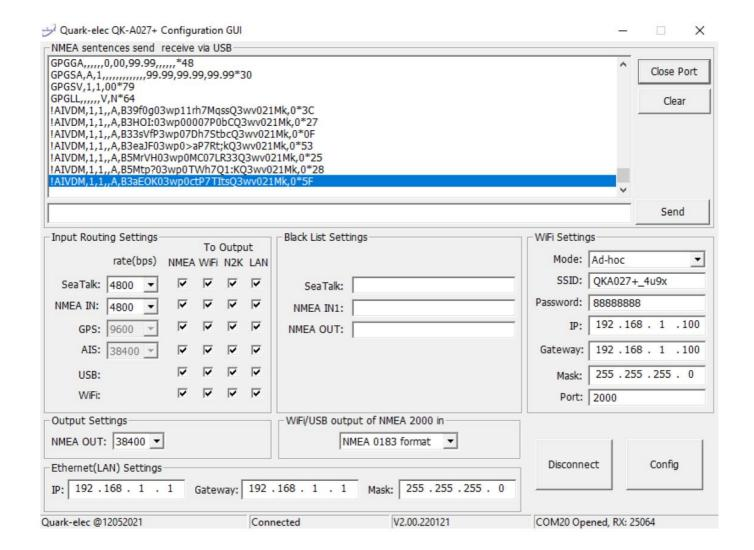
Once open, click 'Connect'. When the A027+ is powered up and successfully connected to a computer (Windows system), the application will display 'Connected' and the firmware version in the status bar (at the bottom of the application). Once you have finished modifying the relevant settings, press 'Config' to save them to the A027+. Then click 'Disconnect' to safely remove your device from the PC. Re-start the A027+ to activate the new settings on your device.
