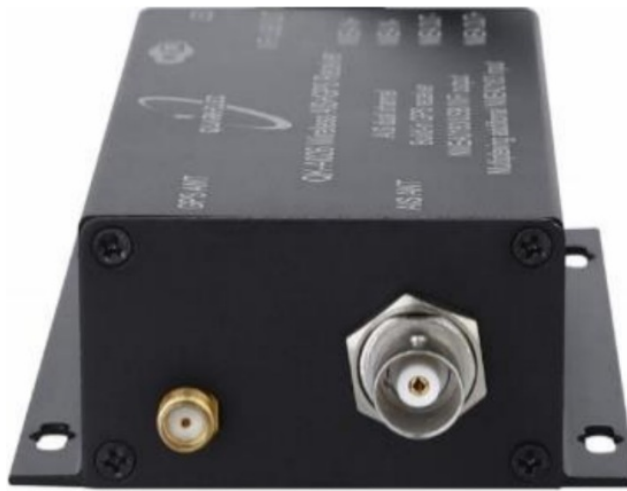
Figure 4: GPS (SMA) and AIS (BNC) antenna connections
