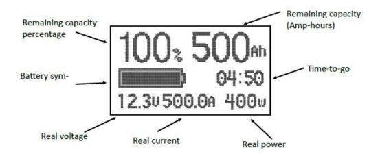
**Remaining capacity percentage:** This shows the percentage of the actual full-charge capacity of the battery. 0% indicates empty while 100% means full.
