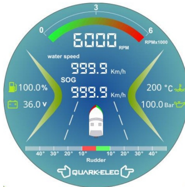
Figure 14 IS10 Rudder Angle Display
