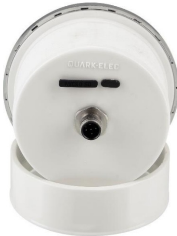
Figure 4 Connectors (back view)
