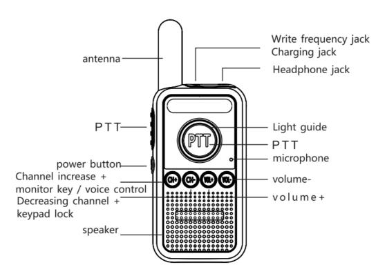
**Switch key:** long press 3S to turn on; long press 3S to turn off.
