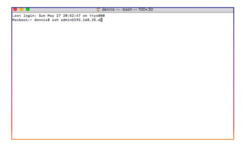
**Step 2:** For first connection to the Access Point using SSH, you may be prompted to accept the host key. Do so by clicking "Yes" and press Enter.
