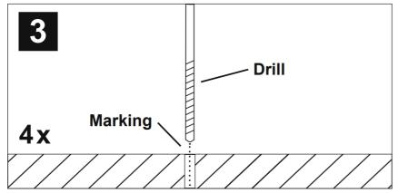
Lay the device aside and then drill the holes for the mounting screws at the marked locations. Please ensure not to damage any components of the vehicle while you drilling the holes. Alternatively (depends on the material of the surface) you can also use self-tapping screws.
