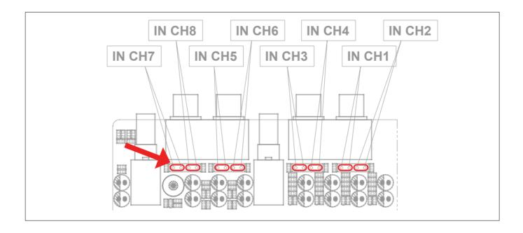
First disconnect the device from the power supply. Then remove the housing cover and locate the six jumpers on the circuit board. These are located below the audio inputs.
