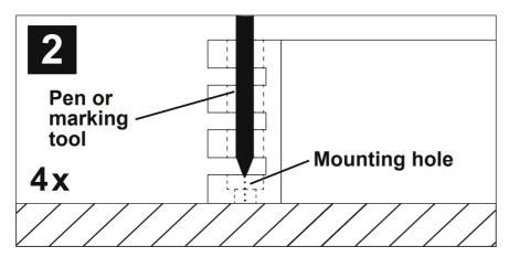
Keep the device at the chosen mounting location in the vehicle. Then mark the four drill holes with an appropriate pen or marking tool through the designated mounting holes at the device.
