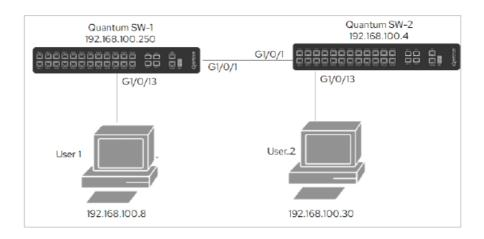
You can observe this network there are two switches are connected user-1 is connected to SW-1 and user-2 is connected to SW-2. For Example, we want to prioritize the ICMP and TCP (video or voice traffic) traffic moving from user-1 to user-2 using cos method.
