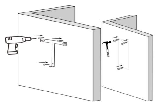
3. Open the cover with the key,fix the charging station with self=tapping screws(3\*M5\*50mm)
