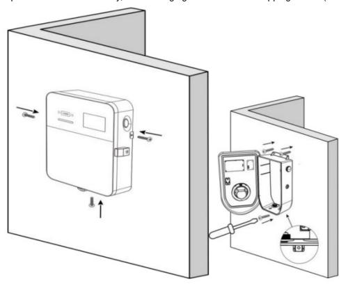
4. Use a cable with a size of 3\*10AWG(32A)/ 3\*9AWG(40A)/ 3\*8AWG(48A)to connect to the input terminal of the charging station, from left to right,N / L and PE wire, and then tighten the screw with a screwdriver.
