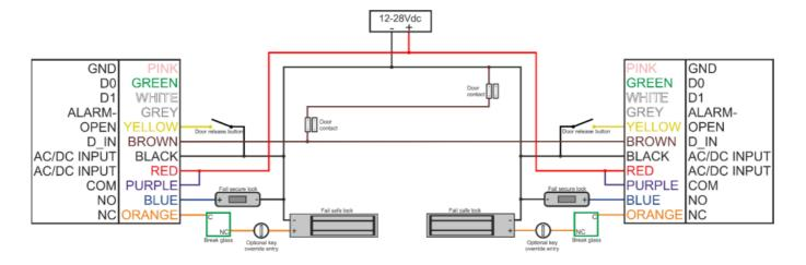
Install IN4004 diodes across the lock +V and -V
