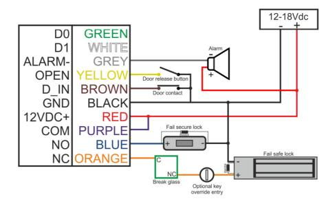
Install IN4004 diode across the lock +V and -V Wiring diagram – Gate, barrier, etc.
