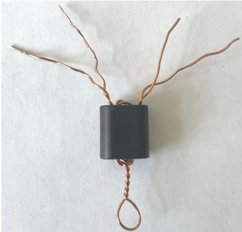
The bottom twisted hairpin loop is the primary, connecting to BS170 transistor drains. Two of the top four wires are the secondary winding, the other two with continuity to the twisted loop are twisted together to form the center tap.
