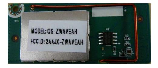
The Qolsys Z-WaveAH Plus Module features the 500 series Z-Wave Wireless Microcontroller silicon from Sigma Designs, providing an air interface to certified Z-Wave devices. OEMs that integrate this module will be able to connect to a variety of smart devices for home automation and control, for example: thermostats, door locks, light bulbs, and electrical outlets. Note: these smart devices must be Z-Wave certified.
