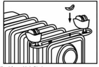
6. Turn the radiator in an upright position after the Castor Wheel Assembly is fitted.
