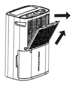
2. Clean Filter: Use a vacuum cleaner to gently absorb dust on filter screen surface. If very dirty, use warm water and gentle detergent. Keep dry.
