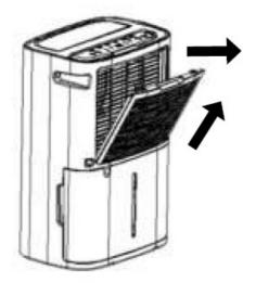
2. Clean Filter: Use a vacuum cleaner to gently absorb dust on the filter screen surface. If very dirty, use warm water and gentle detergent. Keep dry.
