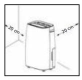
Respect the required distance of the device to walls and other objects.
