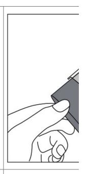
1. Tear off the protective film of the projection lamp piece and fasten it.
