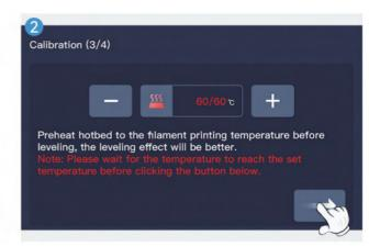
Click the button to initiate the hot bed heating process and set the temperature according to your print filament. Allow the temperature to reach the value and proceed to the next step.
