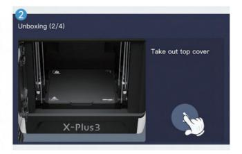
According to the on-screen instructions, remove the top cover from the machine and then click on the next step.
