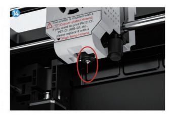
Click the downwards button and allow the filament to emerge from the nozzle.
