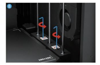
Follow the on-screen instructions to remove the four screws securing the printing platform in place.
