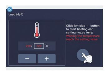
Enter the print temperature for the filament and press the Heat button. Allow the temperature to reach the preset value and then proceed to the next step.
