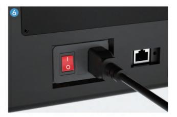
Take out the power cord from the accessory box and plug it into the printer. Turn on the printer and follow the instructions of screen to complete the unboxing process, calibration, etc.
