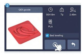
Insert the USB flash drive and select the model inside the test folder for first printing.
