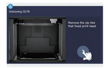
Remove the four ties that secure the platform and proceed to the next step.
