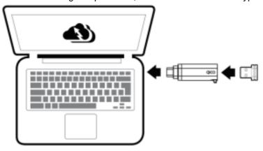
Or Connect the dongle to the USB type-A receptacle of computer.
