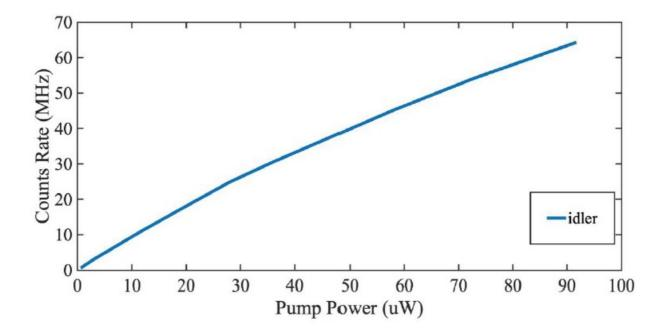
The above figure shows the pump laser power vs the idler intrinsic counts rate, in which the count rate is integrated among all 16 entanglement pairs.
