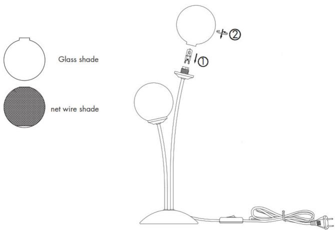
Suitable light source G9, Halogen Max 28W
