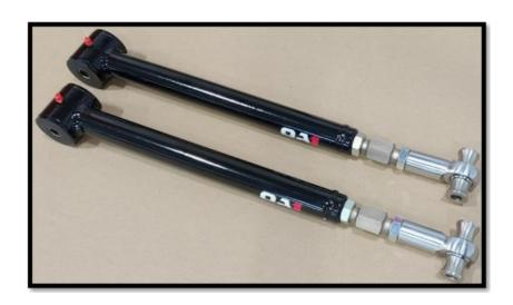
**NOTE:** These trailing arms are shipped at an adjusted length (22" for '71-'96 B-body and 19.25" for '78-'88 G-body which is the factory length for each application. Ensure both trailing arms are at the intended center/center length before beginning the installation.
