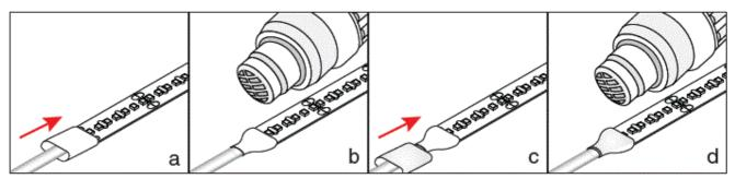
ONCE ALL CONNECTIONS ARE FUNCTIONING PROPERLY, DISCONNECT THE POWER AND BEGIN HEAT SHRINKING INSTRUCTIONS BELOW:
