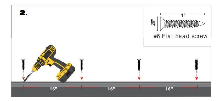
Using pre-drilled pilot holes screw the #6 flat head screws to mount the PPS-BRACKET (1 screw every 16").
