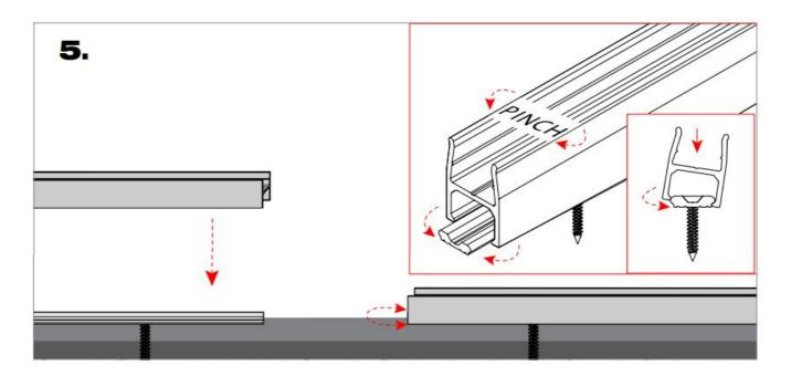
To mount, pinch the upper half of the PPS-96 or PPS-FT while you pivot it around one side of the PPS-BRACKET and push-in until you hear it snap into place. The PPS-96 or PPS-FT flexes around the PPS-BRACKET to create a solid, and secure snap on connection.
