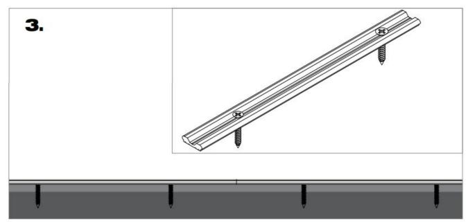
Using pre-drilled pilot holes, use the #6 flat head screws to mount the PPS-BRACKET.
