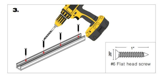
Using pre-drilled holes, use the #6 flat head screws to mount the PPS-LP.
