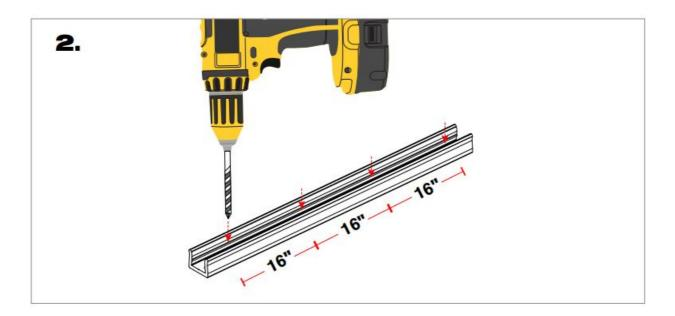
Drill holes (1 hole/screw every 16") into the PPS-LP.
