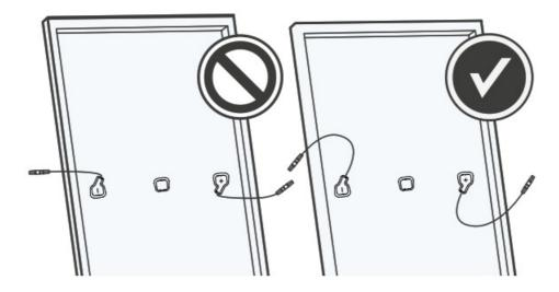
Do not connect modules with different orientations or angles of inclination in the same string.
