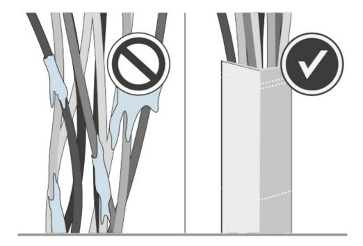
Ensure that the plug connections are secured away from any water-channeling surface.
