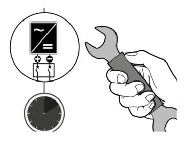
Never plug or unplug the cable when under load. Modules must not carry any current.
