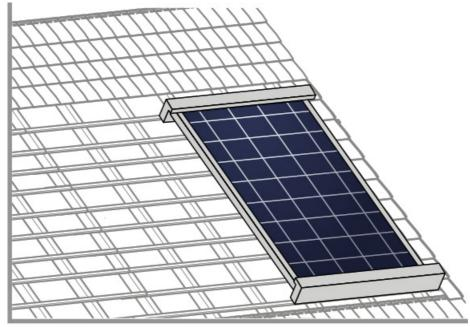
Maintain an interval of at least 0.39 in (10 mm) between two modules along the short side and 0.20 in (5 mm) along the long side.
