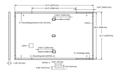
**Fig. 1**: External dimensions (in inch (mm)) and components for Q.PEAK DUO ML-G10, Q.PEAK DUO ML-G10+, Q.PEAK DUO ML-G10.2, Q.PEAK DUO BLK ML-G10, Q.PEAK DUO BLK ML-G10+, Q.PEAK DUO ML-G10.a, Q.PEAK DUO ML-G10.a+, Q.PEAK DUO BLK ML-G10.a and Q.PEAK DUO BLK ML-G10.a+
