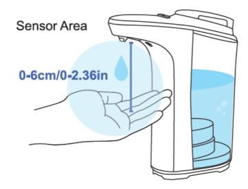
• This unit adopts infrared sensor technology; the optimal sensor range between your hand and the sensor is 0-6cm/0-2.36in.
