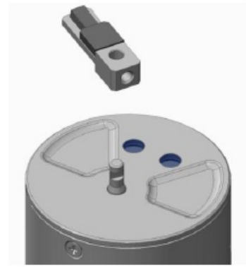
Figure 31 Remove the old wiper arm
