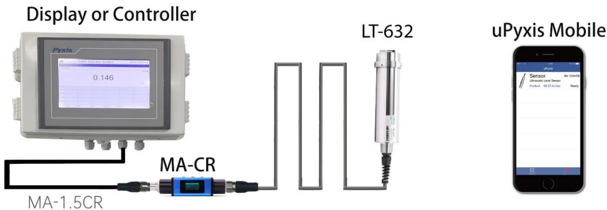
Figure 5 – LT-63X Series Sensor and MA-CR Bluetooth Adapter Powered By Connected Display, Controller or PLC Download and install the uPyxis APP from Apple Store or Google Play per the QR codes provided in the image above. Be sure to turn on Bluetooth in the mobile device (please do not pair the device Bluetooth to any Pyxis device, the uPyxis APP will do the pairing). Open the uPyxis APP in the mobile device. Finger swipe the screen downward to refresh the screen and scan for the available Pyxis Bluetooth devices. The discovered devices will be listed (see Figure 6).
