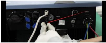
4. Connect the power cable of the energy meter to the grid.
