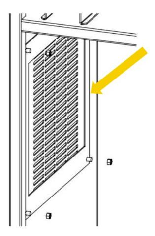
2. Screw the nuts and insert the filter from the gap between the mounting plate and the main body.
