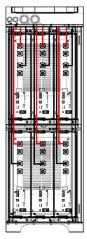
2. Connect the communication cables between batteries as shown in the pic, and connect the host battery with the battery to inverter com cable.
