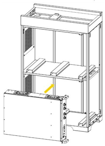
2. Fix the batteries to the main body with screws.
