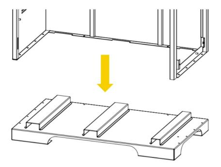
3. Fix the main body and the base by 10 screws.
