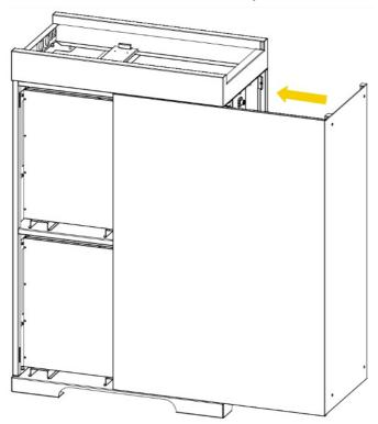
2. Fix the side cover and the main body with screws.
