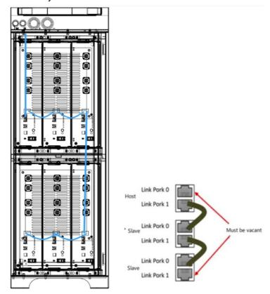
3. Connect the ground wire between the batteries.
