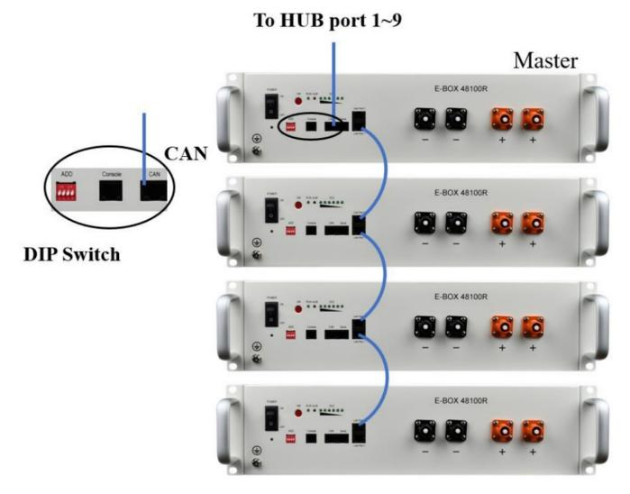
2. Connect the battery groups to the HUB by battery comma cables\*. (See the footnote in the end of the document.)
