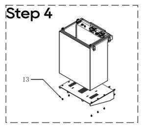
Install the main cabinet to wall by aligning Wall Mounting Adapter to Wall Mounting Plate. Then to fix the main cabinet to Wall Mounting Base with M6 Screws.
