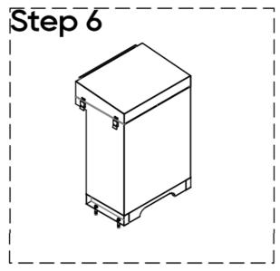
Place and lock the top cover to main cabinet by twisting the latches.
