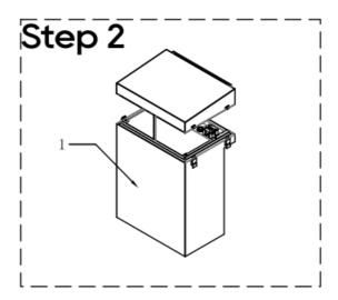
Untwist latches to remove the top cover of main cabinet.
