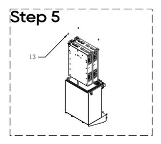
Place the batteries into cabinet as shown in pic- ture and fix them to cabinet with M6 Screws.
