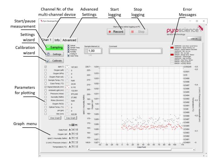
The main window can look differently depending on the type of device you are using. When using a multi-channel device such as FSPRO-4, each channel is individually adjustable and will be shown in the tabs. All channels are controllable simultaneously with an additional control bar. When using devices with stand-alone logging function such as AquapHOx Loggers, a new tab for the logging function will be shown.
