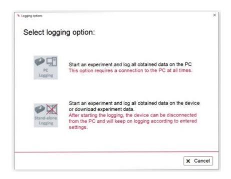
**PC Logging** requires a permanent connection via the USB cable to the PC. The data are not stored on the device, but on the PC.
