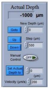
While the motor is moving, the background of the Actual Depth indicator turns red and a red STOP Motor button appears. The motor can be stopped any time by pressing this button. The velocity of the motor can be set in Velocity (range 1-2000  $\mu$ m/s for MU1 and MUX2). The maximum speed should only be used for traveling larger distances. For the actual microprofiling measurements speeds around 100-200  $\mu$ m/s are recommended.
