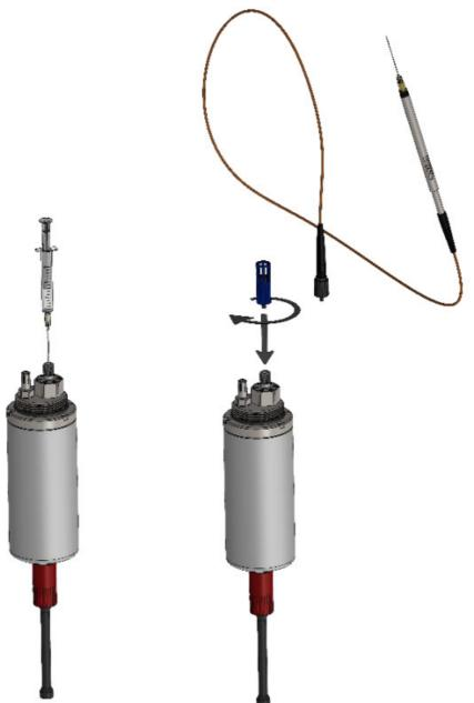
Alternatively, and mandatory for the optical fiber with lens (item no. SPFIB-LNS-SUB/SPFIBLNS-CL2-SUB) for read-out of sensor spots, insert the provided Pasteur pipette to the bottom of the connector and fill with silicone oil.
