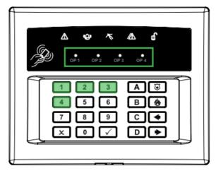
• The OP1-4 LEDs will illuminate once the 1-4 numeric keys have been pressed. Once illuminated, it signifies that the output has been triggered. Press the key again to deactivate the output.
