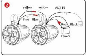
• Step 7: Connected two speakers by RGB connect wire, see the drawing in below (See Illustration 3)
